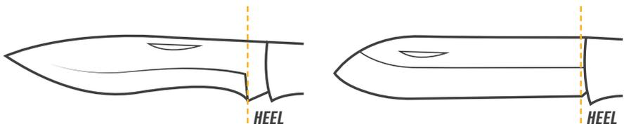
WITH THE MOTOR OFF, POSITION BELT AT THE HEEL OF YOUR KNIVES EDGE.
